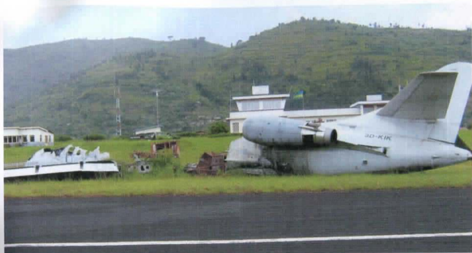
SE210 Caravelle 3D-KIK Gabon Airways Gisenyi, Rwanda 15 November 2005 Last airworthy Caravelle, crashed 28 August 2004 Landed long and hard, starboard undercarriage collapsed and burnt out at Gisenyi, Rwanda No-one was injured and aircraft was a write-off! Peter Horne
