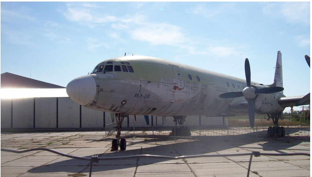
(189001604)/OK-NAA IL-18B WING TIPS REMOVED
