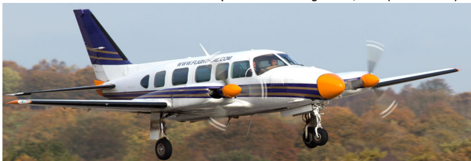
PA-31 G-VIPP calibrating the new glideslope for 14 on 28/10 and 29/10(Robert Burke)
