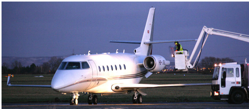
IAI Galaxy HB-JGL being de-iced at Teesside prior to departure, 16/12
