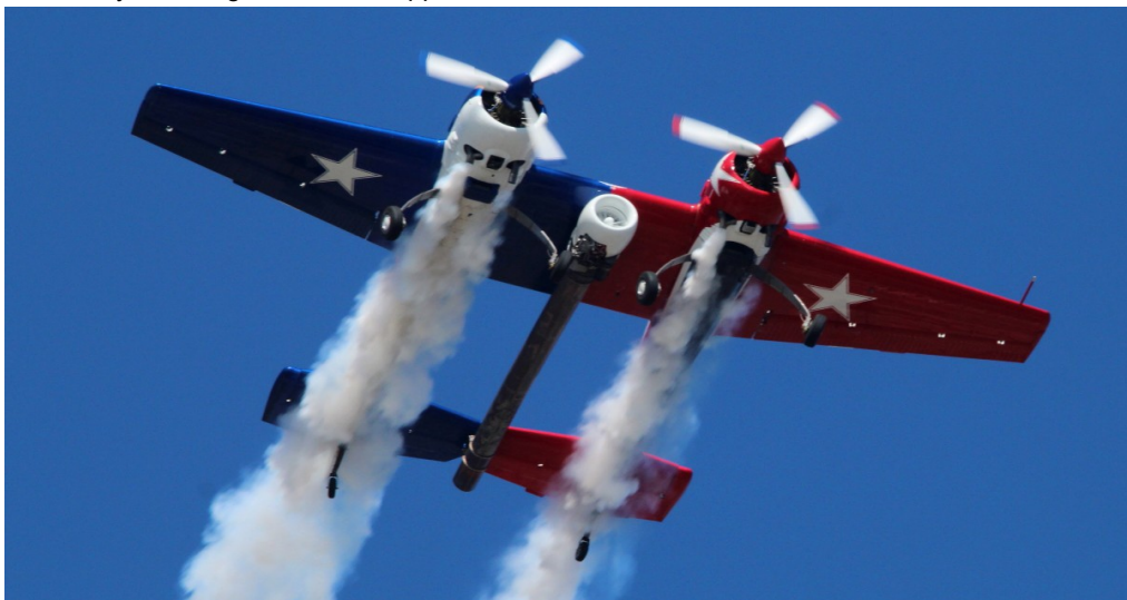
N110JY Yak110 This is actually 2 Yak 55's bolted together with a small jet engine in the middle, N41126 and N955SF
