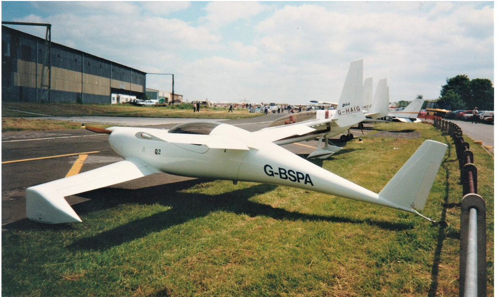
G-BSPA Quickie Aircraft Corporation (QAC) Quickie Q.2. Taken at the Yorkshire Aeroplane Club Fly-in on 29 June 1991. The Q.2 was a kit built composite of fibre-glass, resin and foam. This one dates from 1986. It is a two seat version of the original Rutan Quickie. It has a tandem wing with the elevators on the forward (canard) wing. Note the low level fencing behind the aircraft. Credit: Jim Stanfield
