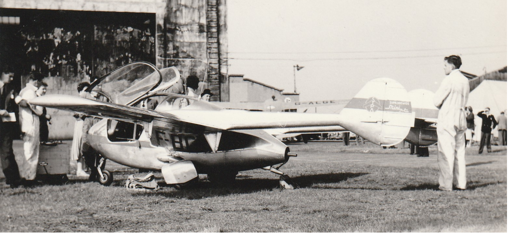
Photograph by Peter Wheatley via David Thompson. F-BGVN Sipa 200 MiniJet. Taken at Yeaton in 1956, in front of the Municipal Hangar, probably at the SSAFA Air Show in May. It was a French designed side-by-side two seater to fulfil the training and liaison role. Wing span of 26 feet and length 17 feet. The first VLJ (Very Light Jet). Only a small number were built (7?) of which this example is No.4. Credit Jim Stanfield
